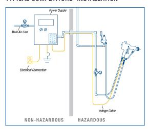
A typical competitors' installation requires a voltage cable that would run between the gun and the power supply located outside the hazardous area. Electrical connections are also required for complete installation.
